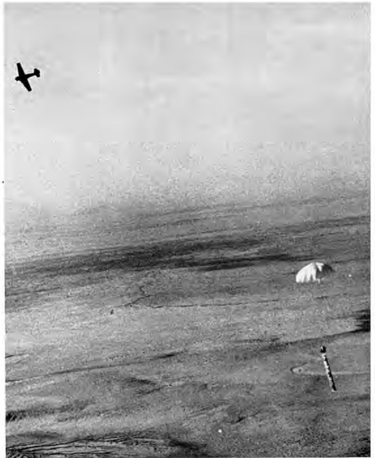
IN TEST DROP over the desert a container holding about 1000 bats is released from plane and floats slowly earthward.
